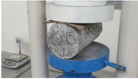
Figure 2: Testing of Split tensile strength
