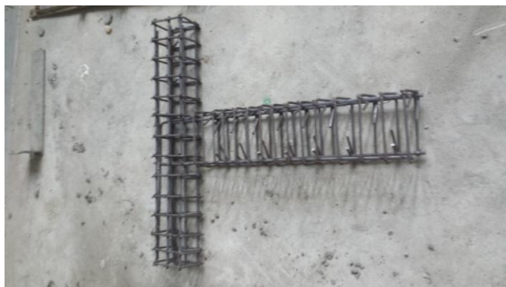
Figure 6: Reinforcement cages for Specimens C1 & C2
