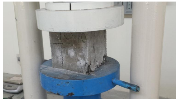
Figure 1: Testing of Compression strength
