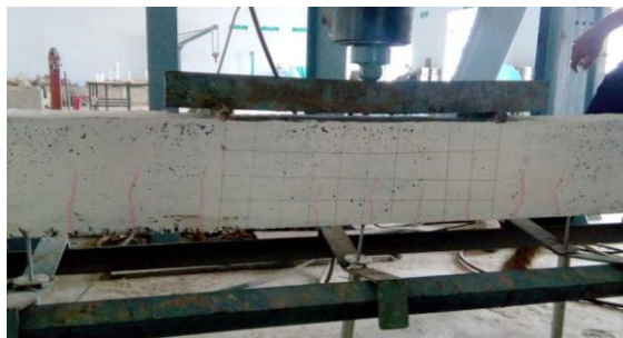
Figure 6. Initial Crack pattern
