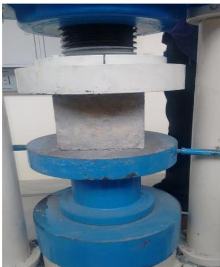
*Figure 1. Compressive strength test*
