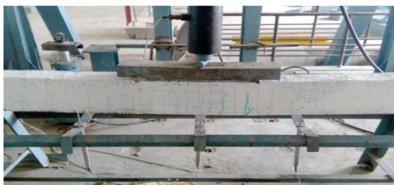
Figure 8. Flexural cracks at Ultimate Load
