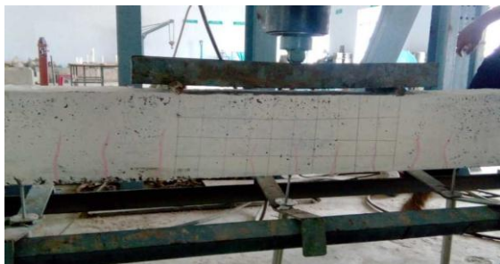
Figure 7. Initial Crack pattern
