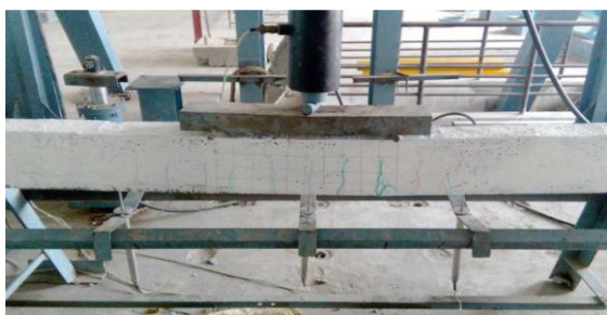
Figure 8. Flexural cracks at Ultimate Load
