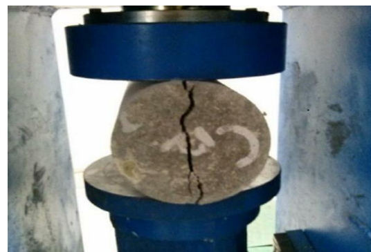
Fig 4: Split Tensile Strength
