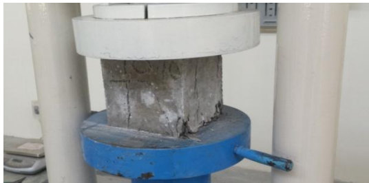
Fig. 2 Compressive Strength Test
