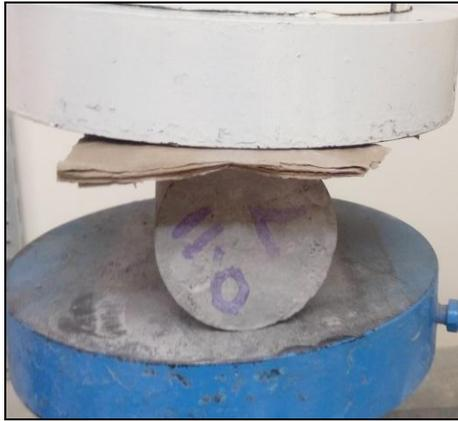
Fig 5.Split tensile test
