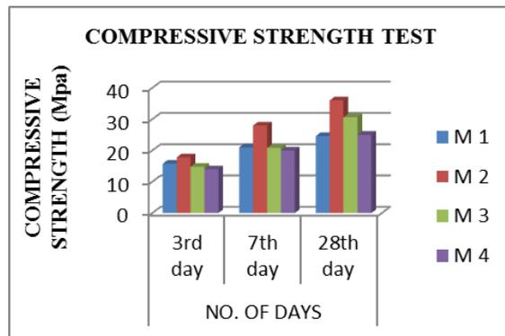
*Fig 4. Compressive Test Graph*
