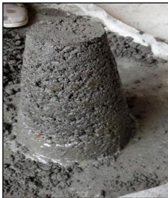
*Fig 2 slump cone*
