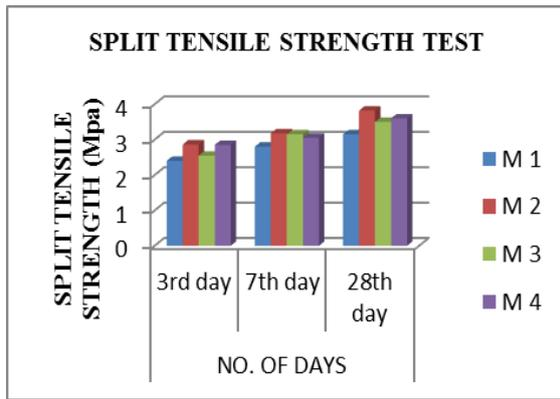
Fig 6.Split Tensile Strength Graph
