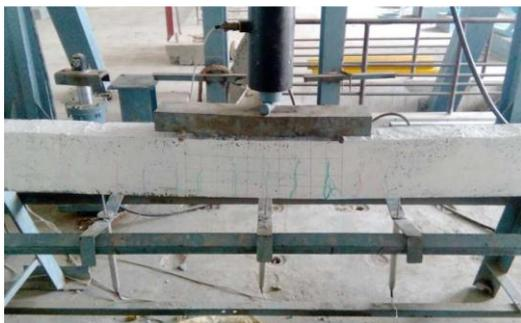
*Figure 6. Flexural cracks at Ultimate Load*
