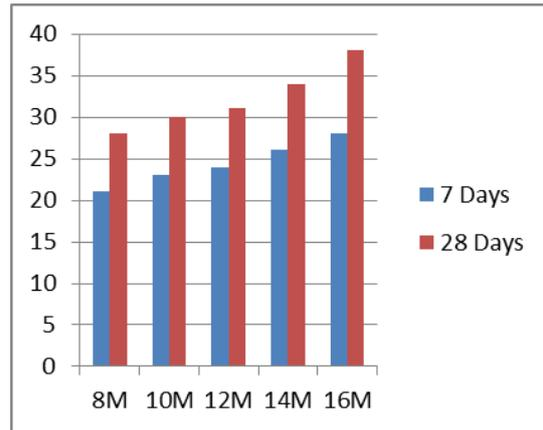
**Figure 2. Chart for compressive strength of SCGC**
