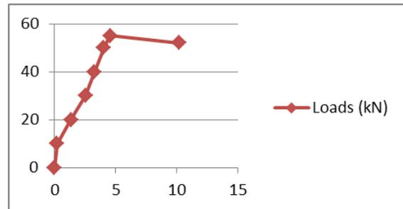
*Figure 7. Load deflection curve plot for NM.*
