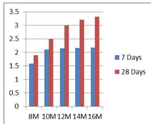
**Figure 4. Chart for compressive strength of SCGC**
