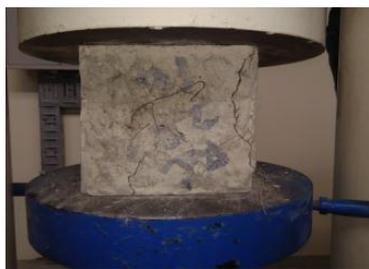
**Figure 1. Compressive strength test**
