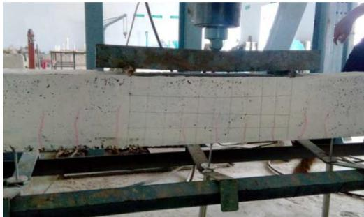
*Figure 5. Initial Crack pattern*
