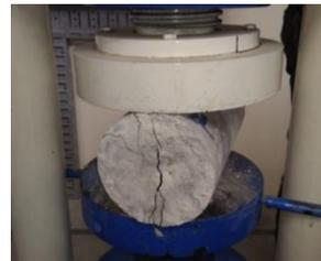
**Figure 3. Split Tensile strength test**
