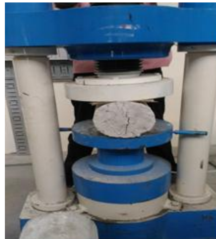
Fig.3 Split Tensile Strength Test
