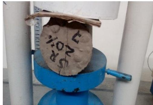
*Fig. 3 Split Tensile Strength Test*
