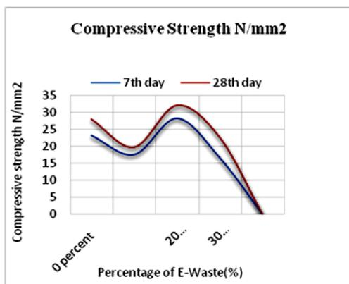
*Fig. 2 Chart for Compressive Strength*
