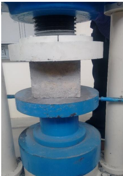
Figure 1. Compressive strength test
