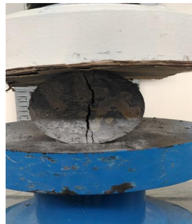
Figure 3. Split tensile strength
