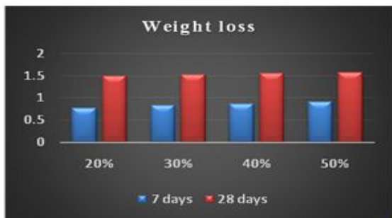
Figure 5. Chart for weight loss percentage of MKPC concrete with fly ash
