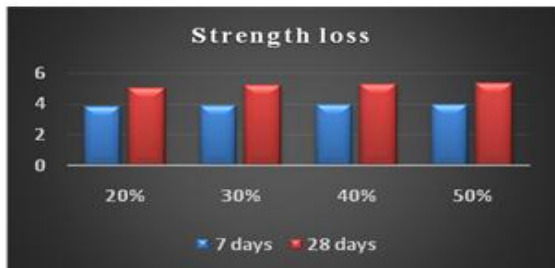
Figure 6. Chart for strength loss percentage of MKPC concrete with fly ash
