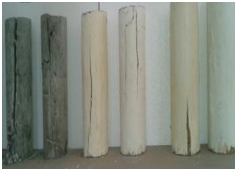
Figure 9: Specimens after Compressive Test
