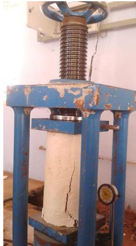
Figure 1: compressive strength test using dial gauge
