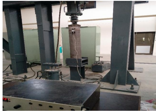
Figure 10: Testing of column in load frame
