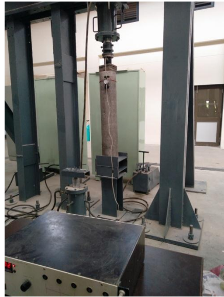
Figure 7. Testing of column in load frame
