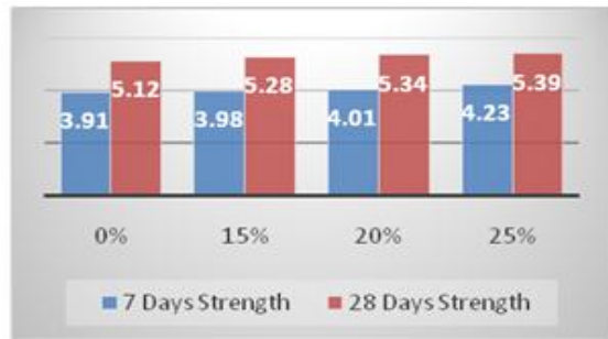
Figure 10: Chart for % strength loss for perlite
