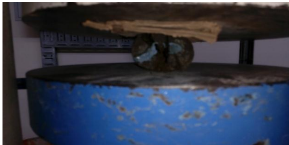
Figure 2: Testing for Split tensile strength
