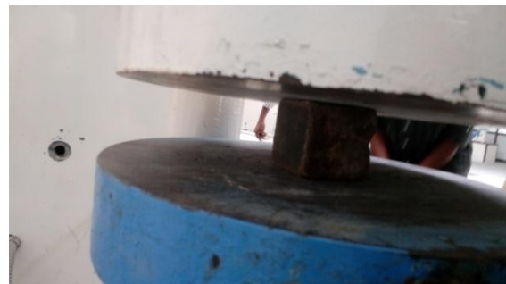
Figure 1: Testing for Compression strength
