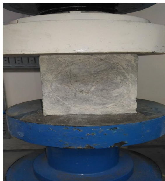
Figure 3 Compressive Strength Test
