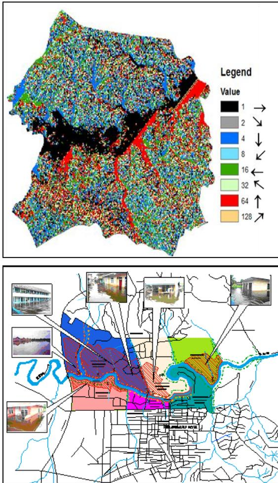
Figure 5 The flow direction and actual flooding
