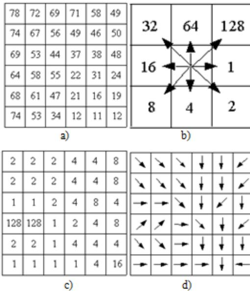
Figure 5 The analysis of flow direction and accumulation using D8 model, a) Elevation b) Flow direction code c) The value of grid d) Arrow symbols of flow direction
