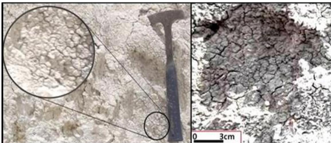
Figure 6 Field photograph showing volcanic expansive soil with ground shrinkage cracks under dry conditions. Length of hammer 32.5cm
