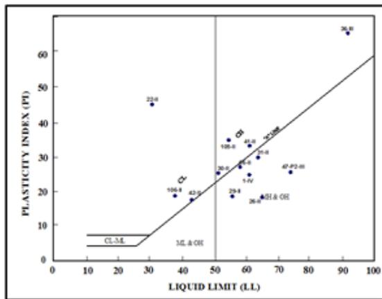
Figure 5. Representation of fine-grained volcanic soils of Taiz city and surrounding on Casagrade plasticity
