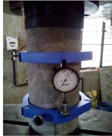
**Figure 1** Setup for modulus of elasticity of concrete
