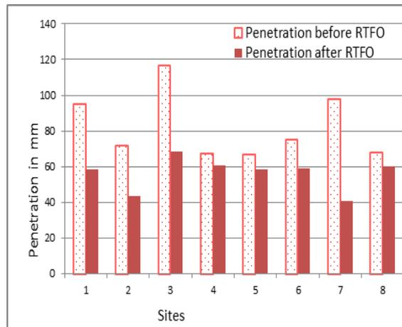
Figure 1 Effect on penetration
