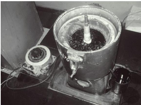
Image 8 Test Set-Up for Bitumen content
