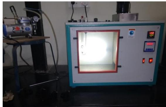
*Image 5 Test Set-Up for viscosity*
