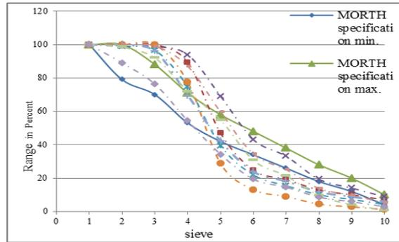
Figure 9 Gradation of asphalt concrete
