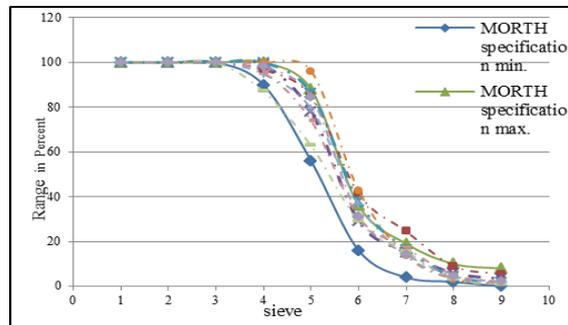
Figure 10. Gradation of bituminous macadam
