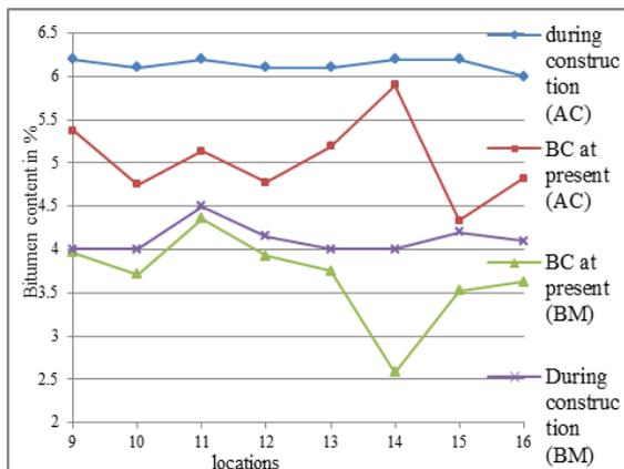
Figure 8 Effect on bitumen content
