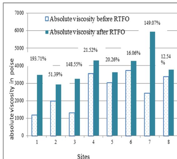
Figure 6 Effect on absolute viscosity
