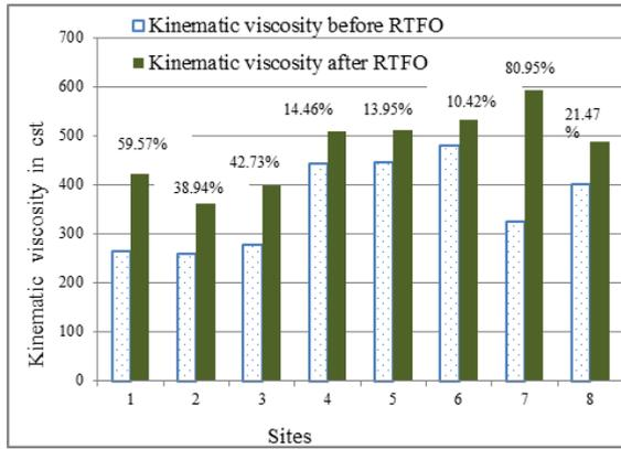
Figure 7 Effect on kinematic viscosity
