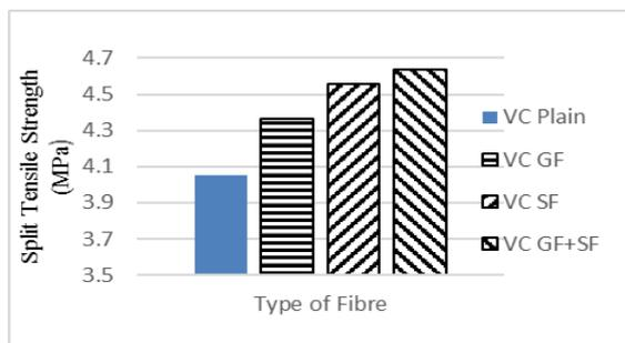
Figure 2(a): Results of split tensile strength of Vibrated Concrete
