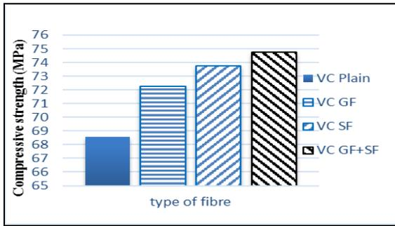
Figure 1(a): Results of compressive strength of Vibrated Concrete
