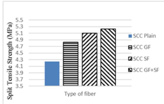
Figure 2(b): Results of split tensile strength of Self Compacting Concrete
