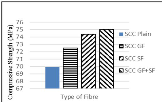
Figure 1(b): Results of compressive strength of Self Compacting Concrete
