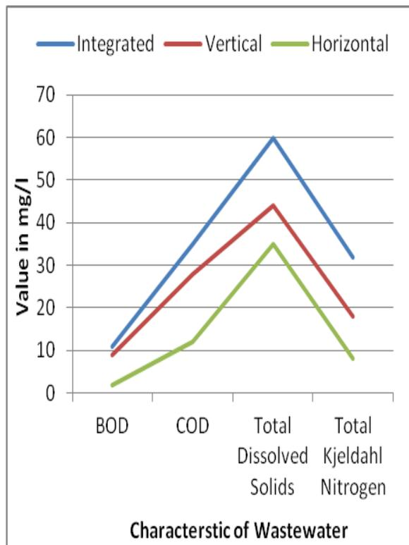
The above bar graph compares average percentage reduction in various characteristics of treated waste water in integrated, vertical and horizontal constructed wetland.
