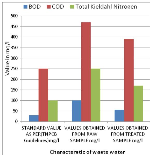
The bar graph represents various characteristic of raw waste water and treated waste water in horizontal constructed wetland as shown in table below.
