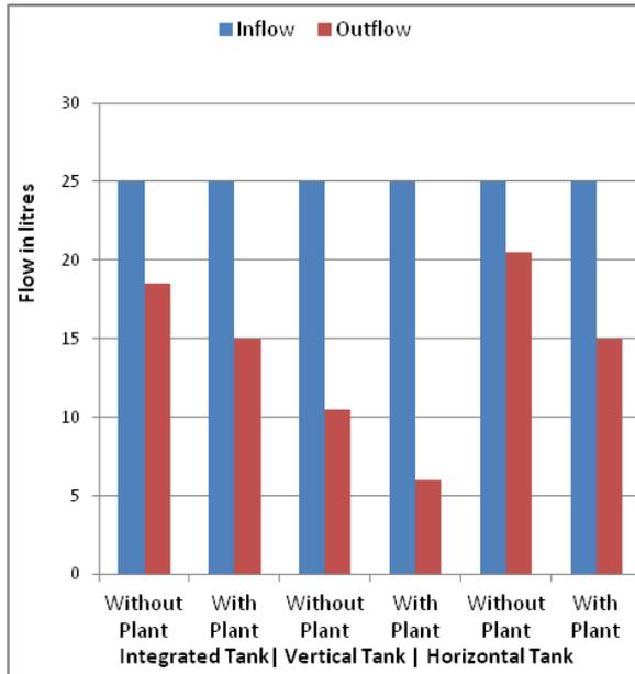
The above bar graph shows total inflow and outflow in litres for various types of constructed wetland. We observe wetland with plant *Typha* have a lower outflow rate.
