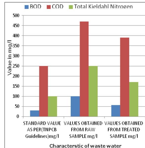
The bar graph represents various characteristic of raw waste water and treated waste water in integrated constructed wetland as shown in table below.
