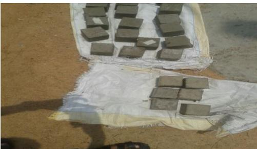
**Fig 4(b): Sun (Atmospheric) curing**
