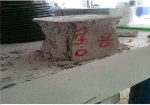
Fig 5(b) failure pattern of specimen
