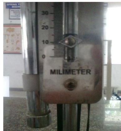
*Fig.2 (b) finale reading of initial setting time*
