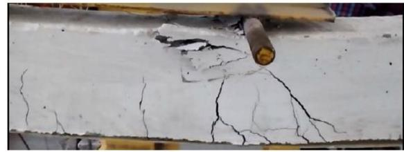
Figure 5 Concrete crushing in AU2
