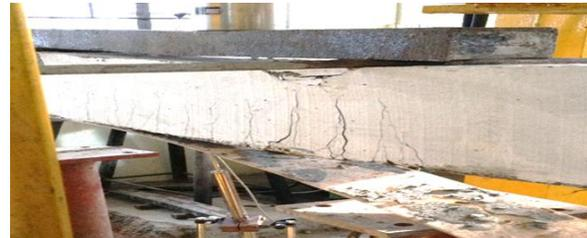
Figure 6 Delamination of FRP in AU2
