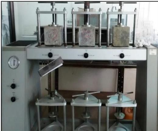
Figure 6 Test setup to determine the depth of Water penetration
