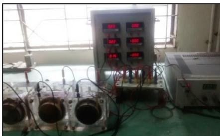
Figure 3 Test setup to determine chloride ion penetration
