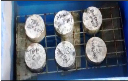
Figure 5 Test setup to determine capillary ingress of water
