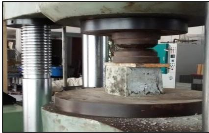
Figure 2 Test setup to determine compressive strength
