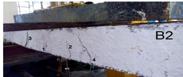
*Fig.11: Failure of the NWC composite beam*
