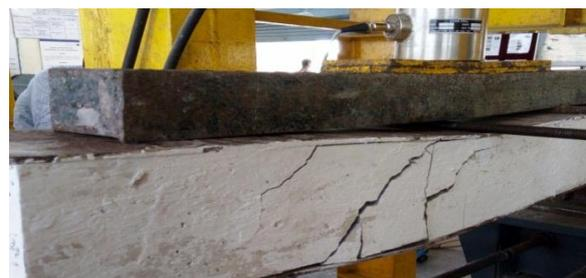
*Fig.13: Shear Failure of the beam at ultimate stage*
