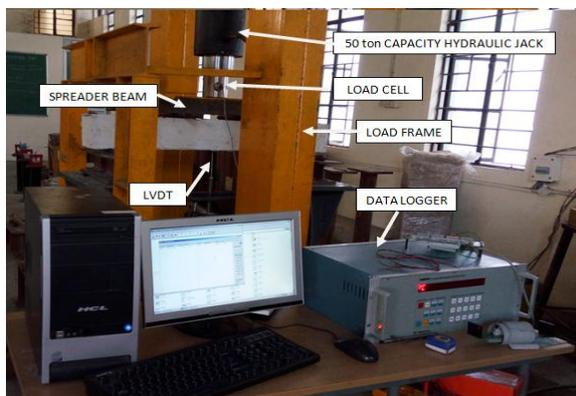
**Fig.7:** Arrangement of the specimens for testing
