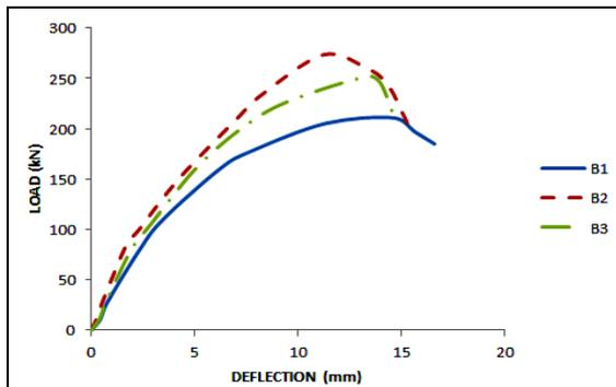
*Fig.9: Load vs Deflection for NWC*
