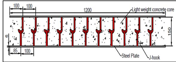
**Fig.4 (a):** Longitudinal section of beam
