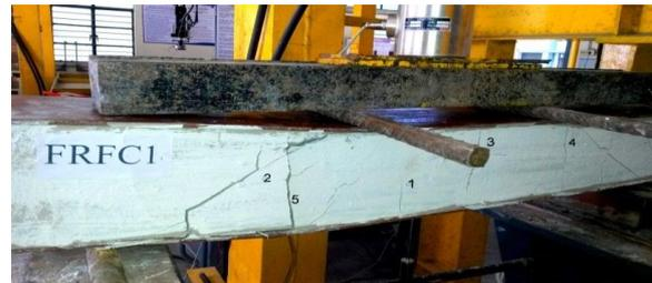
*Fig.12: Failure of LWC composite beams*
