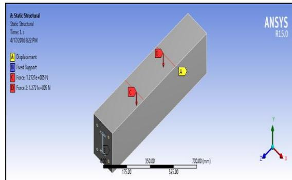
Figure 4 Loading of Beam and Column
