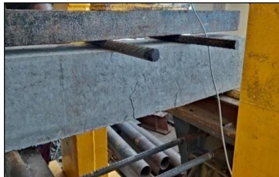
*Figure 8 Failure of B1*
