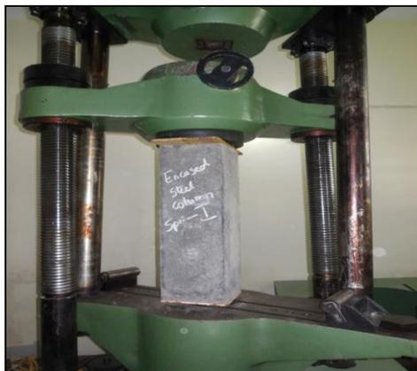
*Figure 7 Test setup for Column*
