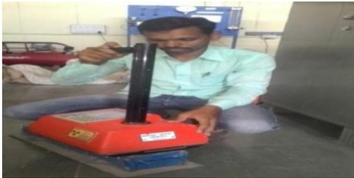
**Figure 1. Measure dry and wet density using nuclear density gauge meter test on beam specimen**
