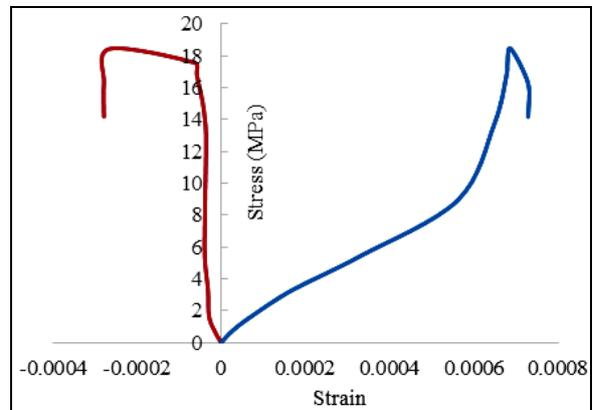
**Figure 6** Stress-Strain behaviour of sandy shale
