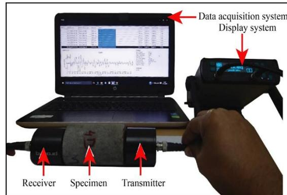
Figure 1 A typical ultrasonic velocity set-up
