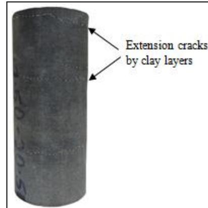
**Figure 3** A water saturated shale sample exhibiting extension cracks along clay layers
