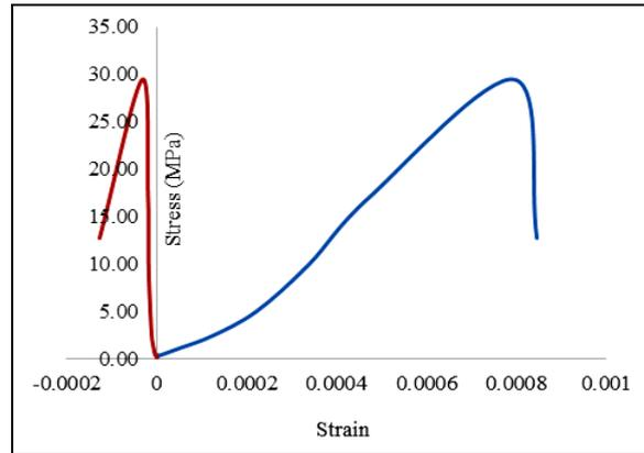
**Figure 5** Stress-Strain behaviour of sandstone
