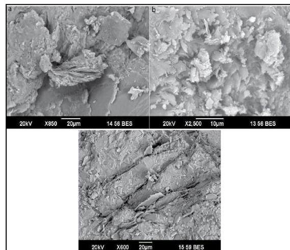
Figure 2 SEM images of (a) sandstone showing flaky clay minerals, (b) sandy shale showing intermediate between sandstone and shale, (c) Shale showing clay minerals occupying cracks along grain boundaries
