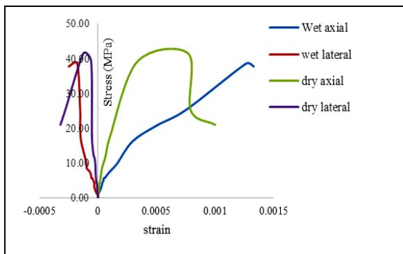
**Figure 4** Stress-Strain behaviour of Shale under dry as well as saturated condition
