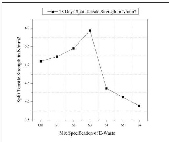
Figure 3 Split tensile strength in  $N/mm^2$
