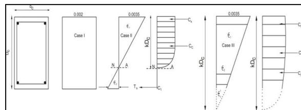
Figure 2 Strain distributions in column section
