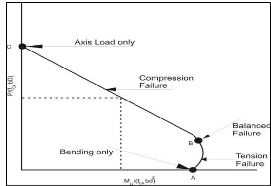
Figure 1 P-M interaction diagram for column
