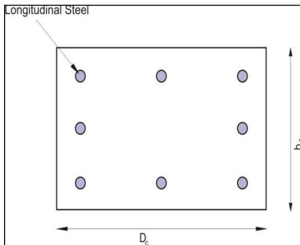
Figure 3 Generalized sectional view of column
