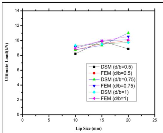
Figure 7 Ultimate load vs lip size for L=2000mm
