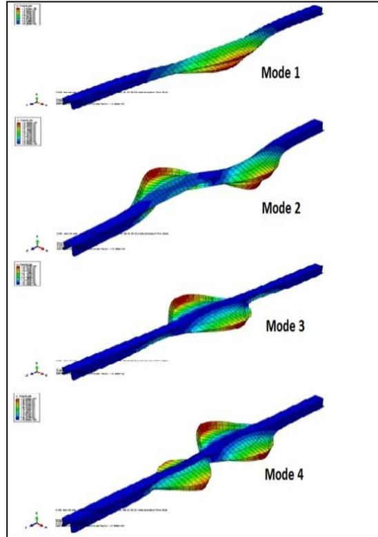
Figure 5 Elastic buckling modes from ABAQUS
