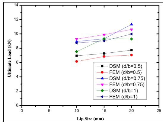
Figure 9 Ultimate load vs lip size for L=3000mm
