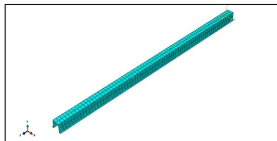
Figure 3 Assembled and meshed model
