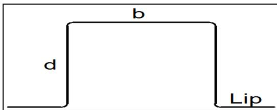
Figure 1 Cross section of hat shaped beam
