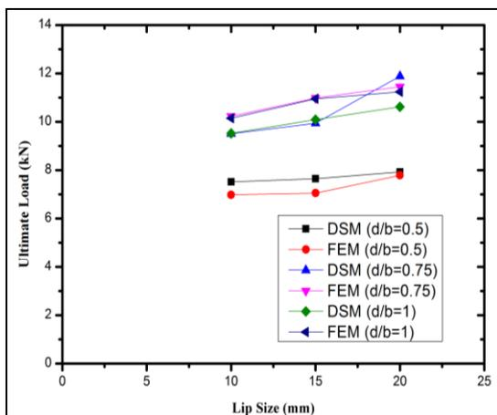
Figure 8 Ultimate load vs lip size for L=2500mm
