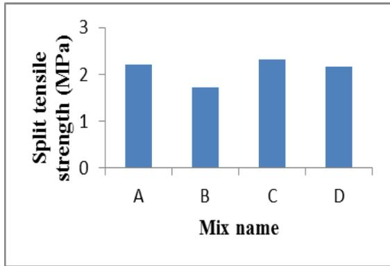
Fig 6 Shows the Split Tensile Strength of Mortar Mix at 28 days
