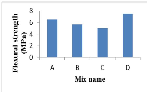
Fig 7 Shows the Flexural Strength of Mortar Mix at 28 days
