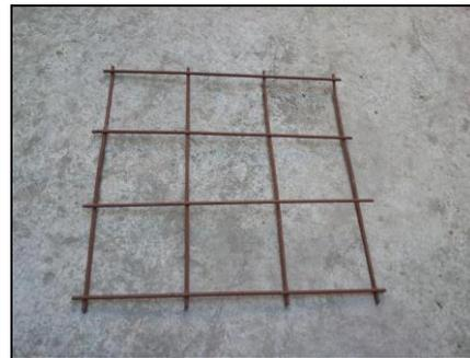
**Fig 2 Weld mesh (60mm x 60mm)**
