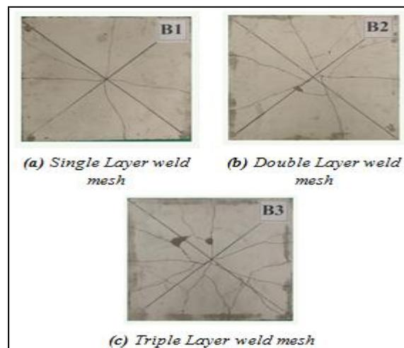
Fig 10 Failure Pattern of Ferrocement slabs with addition of 10% Fumed Silica
