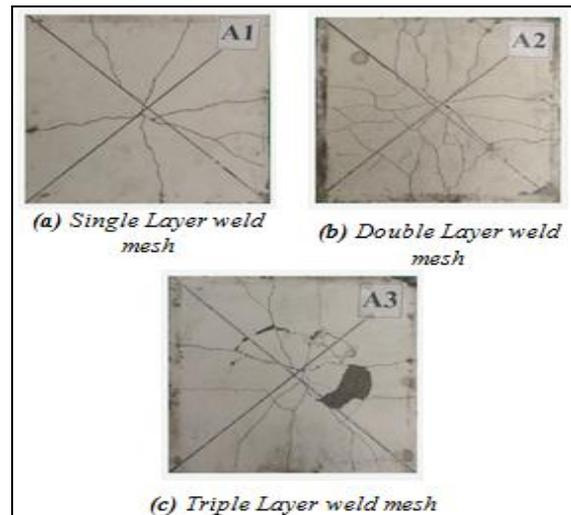
Fig 9 Failure Pattern of Ferrocement slabs of Control Mix
