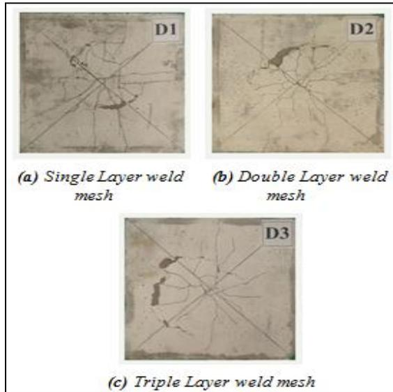
**Fig 12** Failure Pattern of Ferrocement slabs of 40% replacement of cement by GGBS and addition of 10% Fumed Silica
