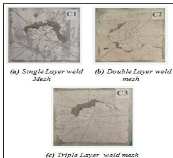
Fig 11 Failure Pattern of Ferrocement slabs of 30% replacement of cement by Fly ash and addition of 10% Fumed Silica
