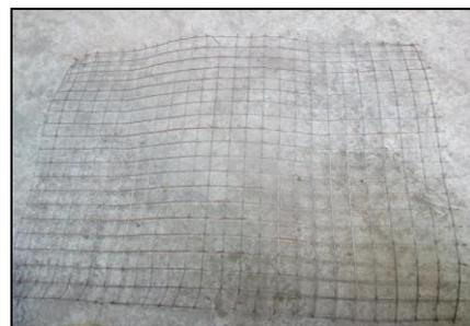
**Fig 3 Wire mesh (10mm x 10mm)**
