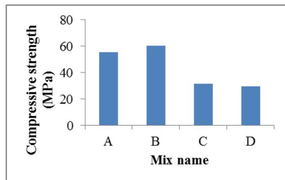
**Fig 5** Shows the Compressive Strength of Mortar Mix at 28 days
