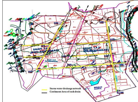
**Figure 4:** Storm water drainage network derived from DEM
