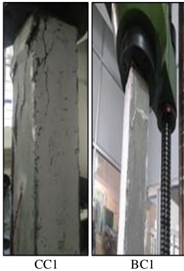
Figure 7 Crack patterns observed in CC1 and BC1
