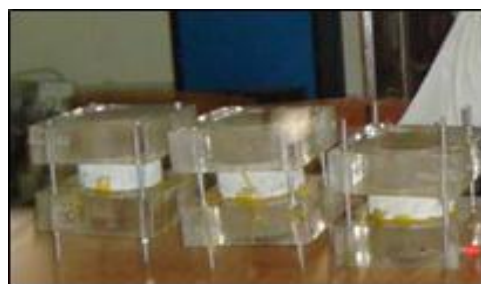
Figure 3 Test setup to determine rapid chloride penetration
