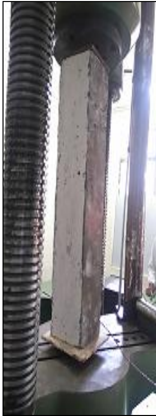
Figure 5 Test setup for column
