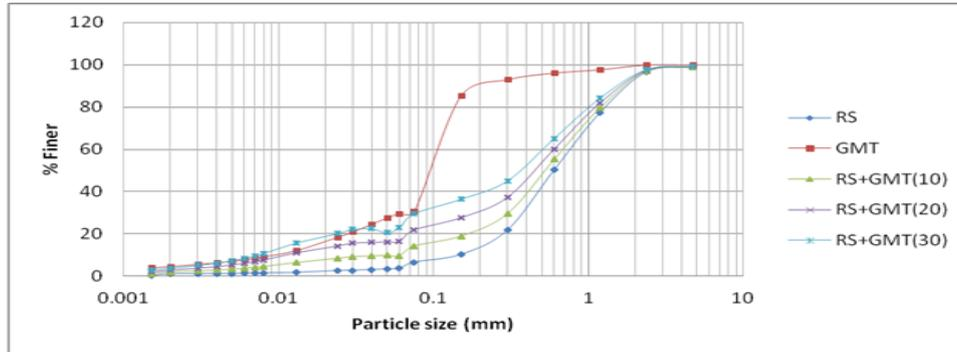
Figure 2. Particle size distribution curves for replacement of river sand with gold mine tailings
