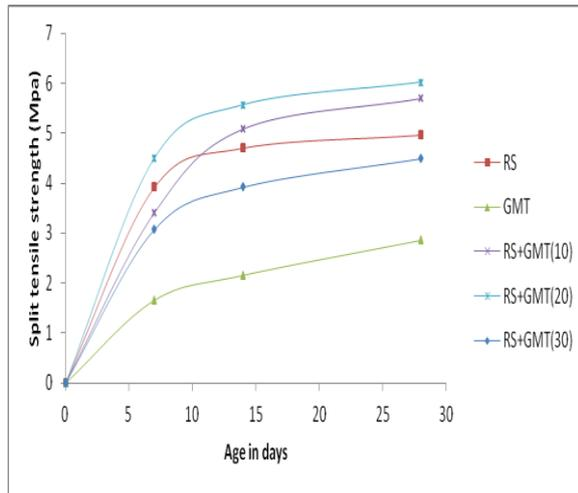
Figure 4 Variation of splitting tensile strength with age
