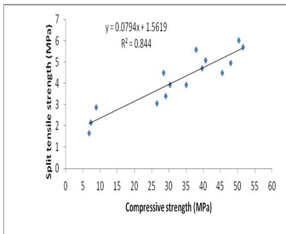
Figure 5 Splitting tensile strength versus compressive strength
