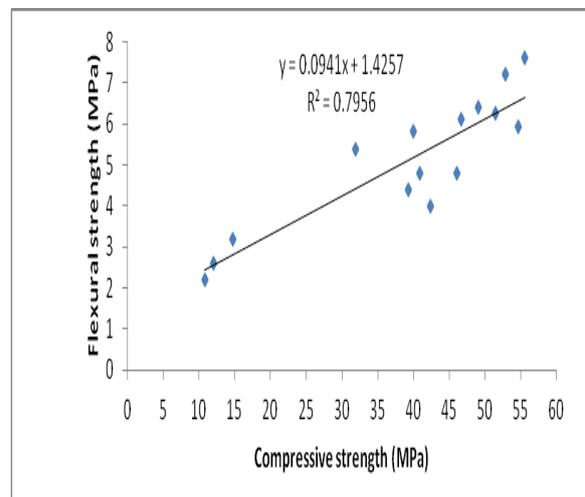
Figure 7 Flexural strength versus compressive strength
