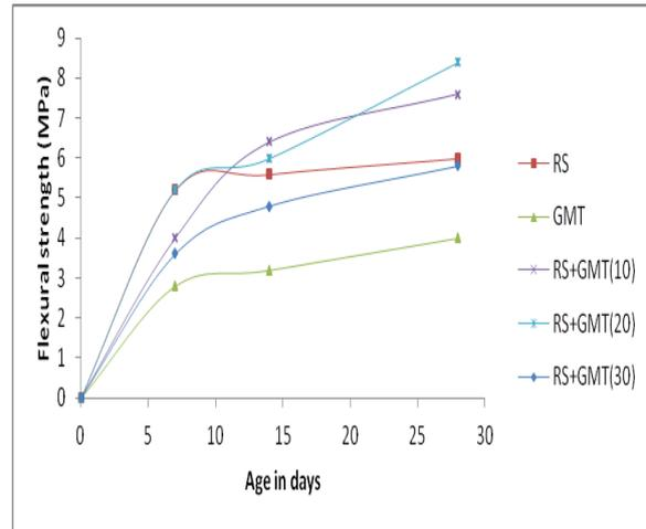
Figure 6 Variation of flexural strength with age
