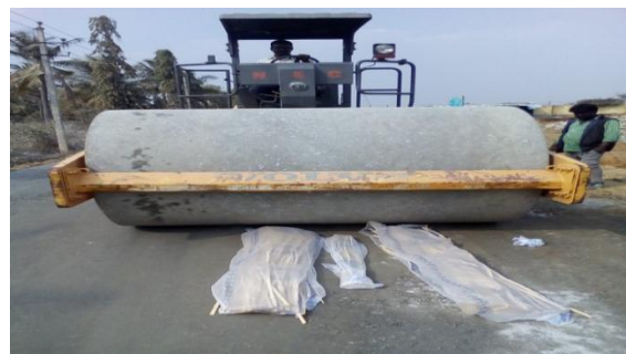
Figure 3 Longitudinal striped bamboo under roller
