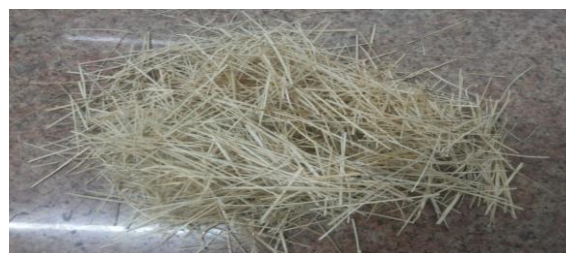
Figure .4 Bamboo fiber of diameter 1.156mm Of aspect ratio (l/d) 40
