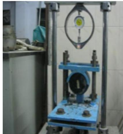
*Image 3 Test set-up for bond strength*
