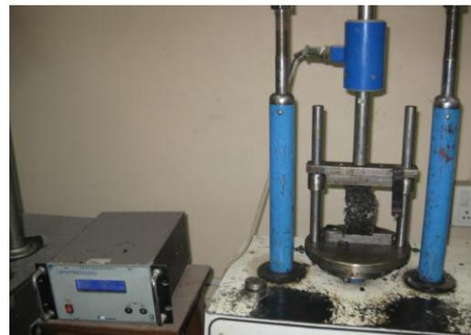
*Image1. Test setup for indirect tensile strength test*
