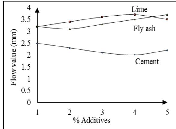
**Figure 2 Flow value v/s % additive**
