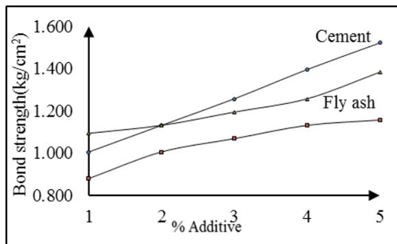
Figure 4. Bond strength v/s % additive
