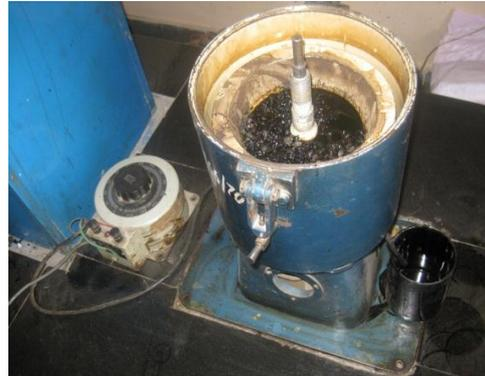
*Image 2. Test set-up for binder content*
