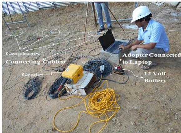
**Figure 1** Single geode test setup and sources at different position
