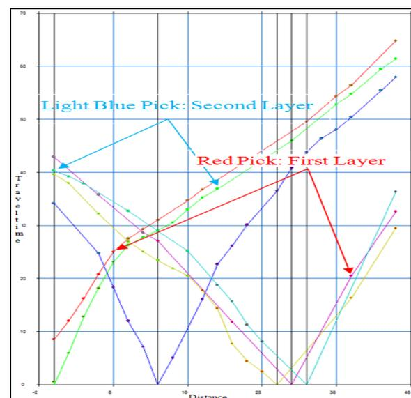
**Figure 2** Travel time curve and layer assignments for B-type quarters
