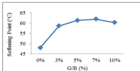
**Figure 3: Softening Point of various Gondorukem in Bitumen**
