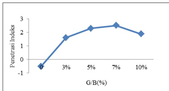
**Figure 4:** Penetration Index of various Gondorukem in Bitumen
