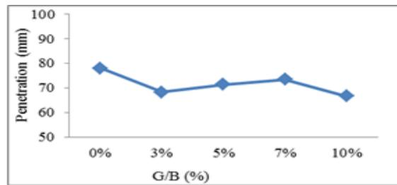
**Figure 2: Penetration value of Gondorukem/Bitumen**
