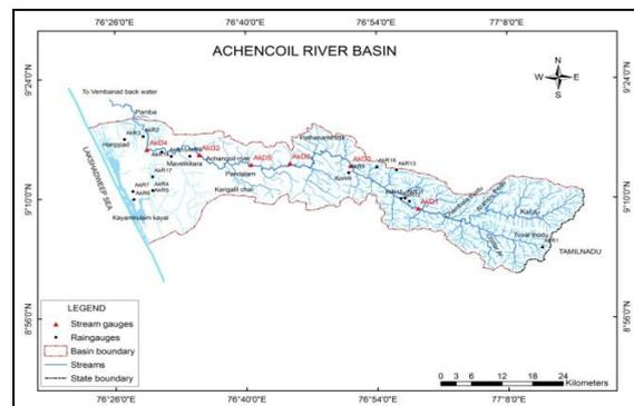
Figure 2 Locations of rain gauge stations and discharge stations in Achencoil river basin
