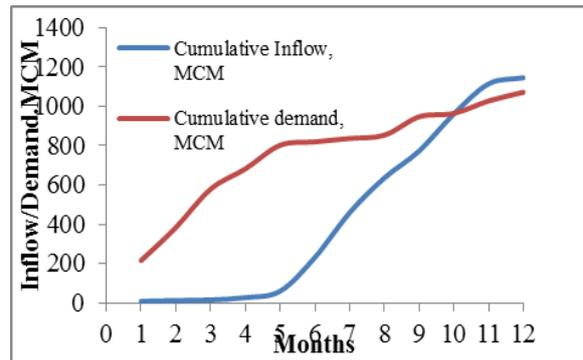
**Figure 10 Mass curve for Achencoil river basin**
