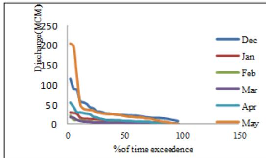
Figure 8 flow duration curves for Thumbabam
