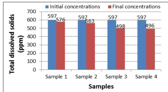
Figure 8 Comparison of initial and final concentration of total dissolved solids using acid treated amla as an adsorbent material
