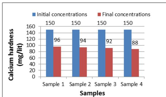
**Figure 10** Comparison of initial concentrations and final concentrations of calcium hardness using acid treated amla powder as an adsorbent material
