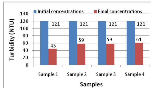
**Figure 3** Comparisons of initial and final concentration of turbidity using oven dried curry leaves as an adsorbent material
