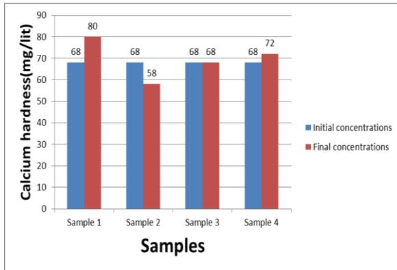
Figure 6 Comparison of initial and final concentration of calcium hardness using oven dried curry leaves as an adsorbent material
