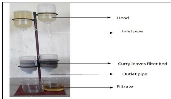
**Figure 2** Filter model with oven dried curry leaves powder as filter bed
