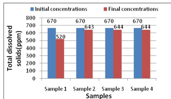
**Figure 4** Comparison of initial and final concentration of total dissolved solids using oven dried curry leaves as an adsorbent material.
