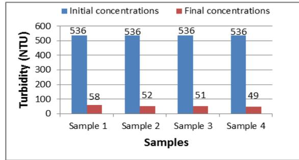
Figure 7 Comparison of initial and final concentration of turbidity using acid treated amla powder as an adsorbent material
