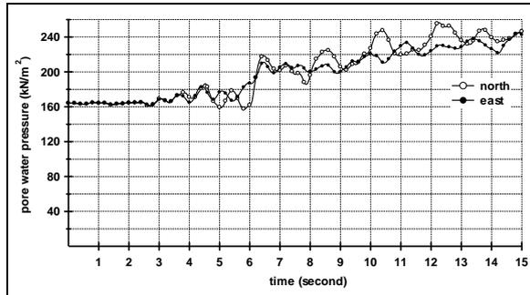
**Figure 8** Time History of the Pore Water Pressures Acting at Beneath of the Waterfront Structure
