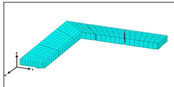
Figure 2 Mesh Partition of Finite Element Seawater Model
