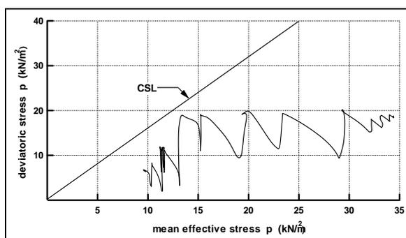
**Figure 10** Effective Stress Path at Behind of the East Waterfront Structure
