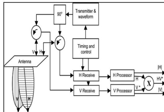
**Fig 9: Hybrid polarity SAR architecture of RISAT -1 (First EO Spacecraft)**
