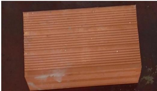
**Fig-2** Showing the data Porotherm blocks of the size 400\*100\*200
