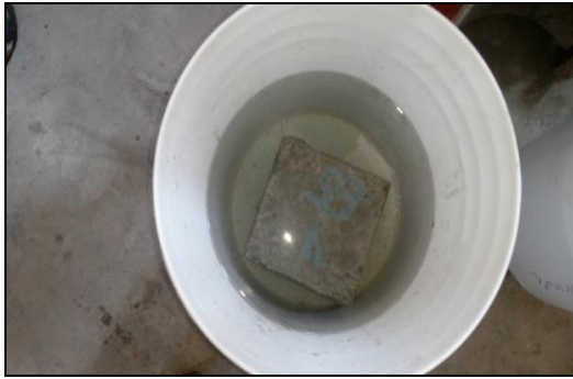
Figure 6 Sulphate Attack Test
