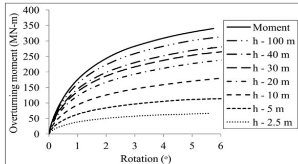
**Figure 4** Overturning moment-rotation plot for bucket foundation in medium dense sand ( $D = 12$  m,  $L = 12$  m,  $V = 10$  MN)
