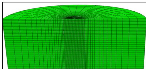
*Figure 1 Discretized model of bucket foundation embedded in medium dense sand (D = 12 m, L = 12 m, V = 10 MN)*
