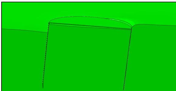
**Figure 2(b).** Enlarged view of deformed configuration of bucket foundation at failure ( $D = 12$  m,  $L = 12$  m,  $V = 10$  MN)
