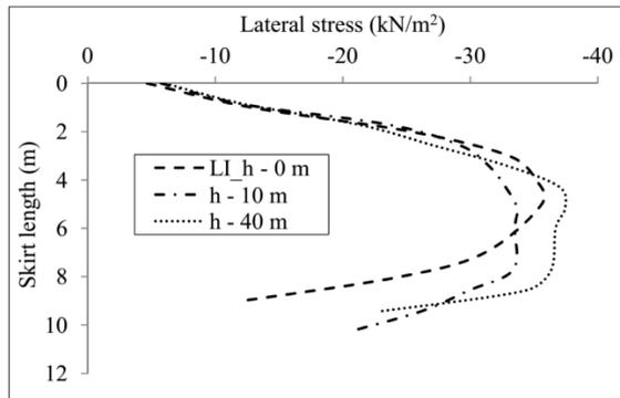
Figure 6(b). Lateral stress along left interior surface of bucket ( $D = 12\text{ m}$ ,  $L = 12\text{ m}$ ,  $V = 10\text{ MN}$ )
