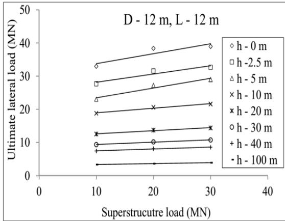
Figure 8 Variation of ultimate lateral capacity with superstructure load
