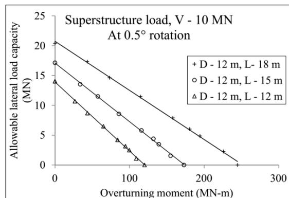
Figure 11(b). Lateral load-overturning moment interaction diagram at 0.5° rotation
