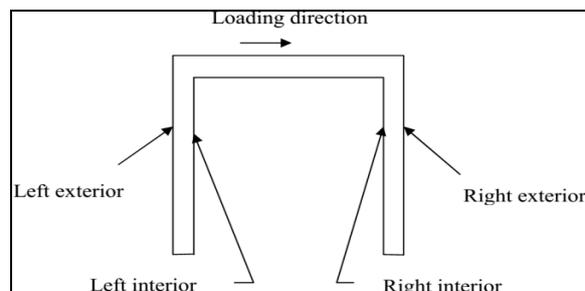
**Figure 5** Schematic diagram representing length in terms of four different location for lateral stress determination
