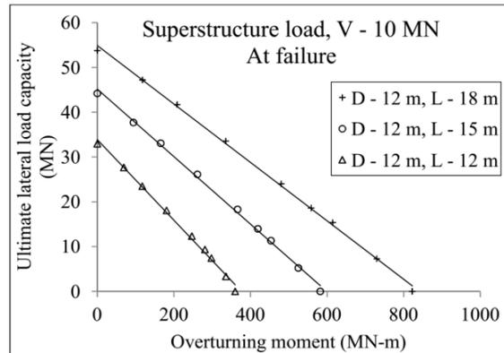
Figure 11(a). Lateral load-overturning moment interaction diagram at failure
