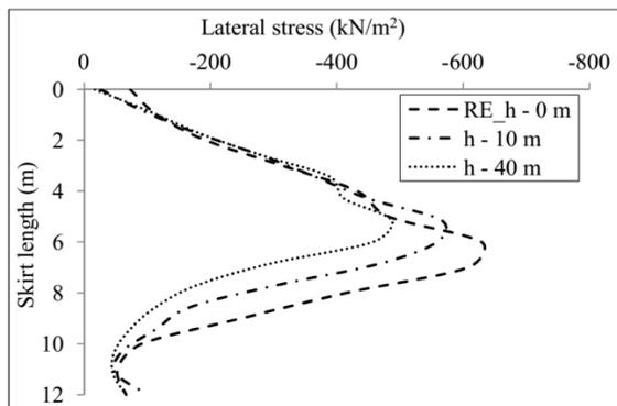
Figure 6(c). Lateral stress along right exterior surface of bucket ( $D = 12\text{ m}$ ,  $L = 12\text{ m}$ ,  $V = 10\text{ MN}$ )
