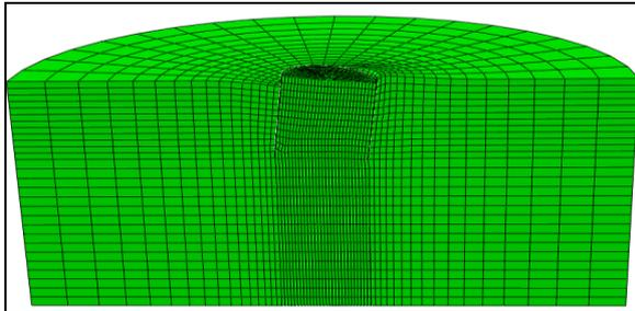
**Figure 2(a).** Deformed configuration of bucket foundation at failure ( $D = 12$  m,  $L = 12$  m,  $V = 10$  MN)
