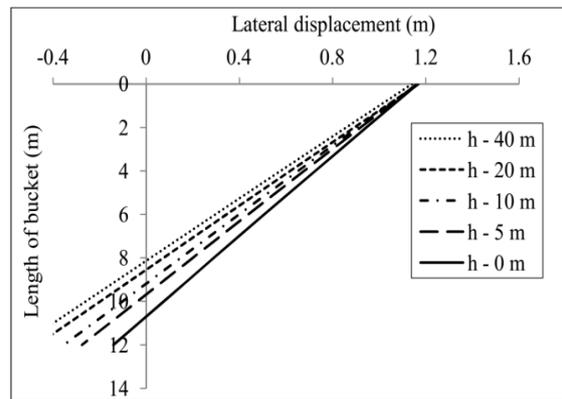
Figure 7 Variation of lateral displacement at right exterior surface of bucket foundation with eccentric loading ( $D = 12\text{ m}$ ,  $L = 12\text{ m}$ ,  $V = 10\text{ MN}$ )
