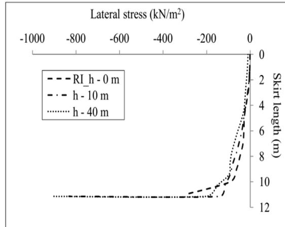
Figure 6(d). Lateral stress along right interior surface of bucket ( $D = 12\text{ m}$ ,  $L = 12\text{ m}$ ,  $V = 10\text{ MN}$ )
