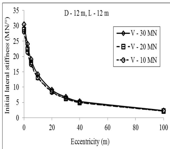
Figure 9 Effect of superstructure load on initial stiffness
