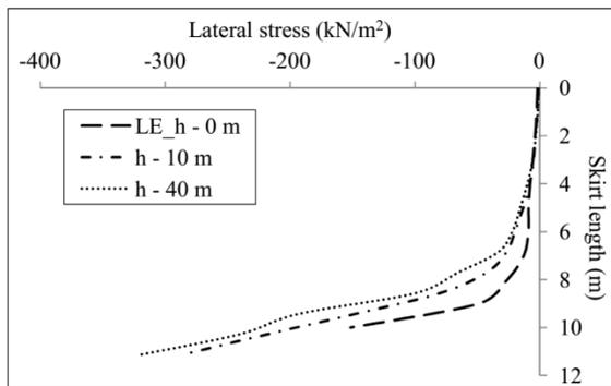
Figure 6(a). Lateral stress along left exterior surface of bucket ( $D = 12\text{ m}$ ,  $L = 12\text{ m}$ ,  $V = 10\text{ MN}$ )
