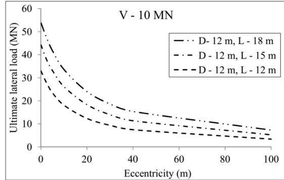
Figure 10 Effect of bucket length on lateral capacity of bucket foundation
