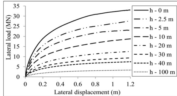
**Figure 3** Lateral load-displacement plot for bucket foundation in medium dense sand ( $D = 12$  m,  $L = 12$  m,  $V = 10$  MN)
