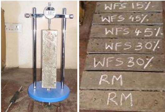
**Figure 6** Drying shrinkage test setup. A) Length comparator B) Prism specimens
