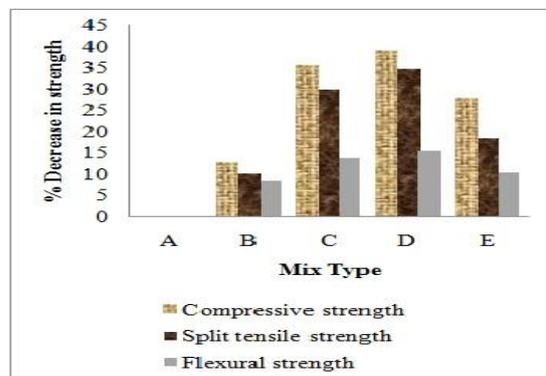
**Figure 4.** Percent decrease in concrete strength at 28 days with respect to control mix
