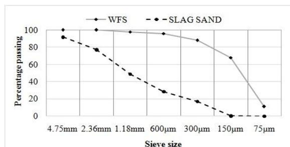
**Figure 2** Particle size distribution of WFS and slag sand
