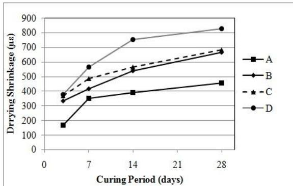
**Figure 5** Drying shrinkage of concrete containing WFS
