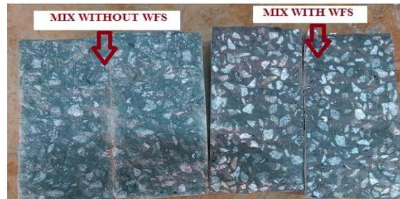
**Figure 3** Failure surface of concrete with and without WFS
