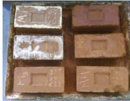
Figure 1 Formation of salts over the surface of Red Mud bricks
