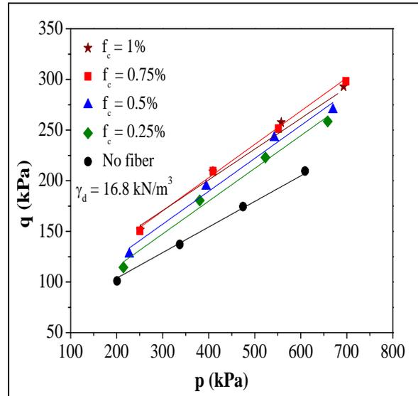
Figure 5 Effect of fiber content on modified failure envelope of fiber-reinforced soil
