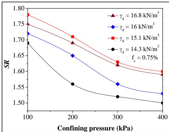
Figure 4 Effect of dry unit weight on SR at different confining pressure
