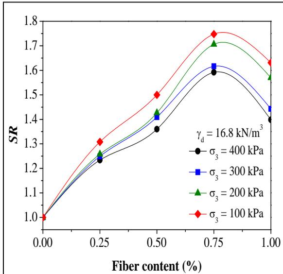
Figure 3 Effect of fiber content on SR at different confining pressures
