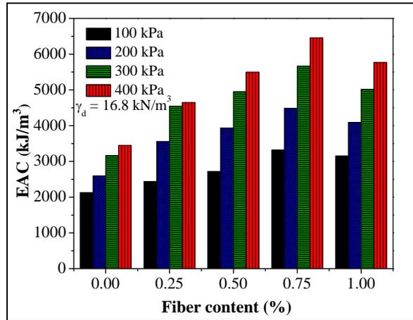
Figure 11 Effect of fiber content on EAC
