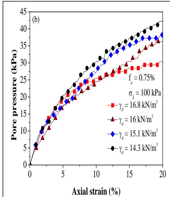
Figure 2 Effect of dry unit weight on (a) stress-strain and (b) pore pressure response
