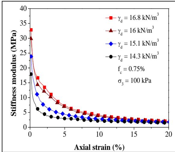
Figure 10 Effect of dry unit weight on stiffness modulus
