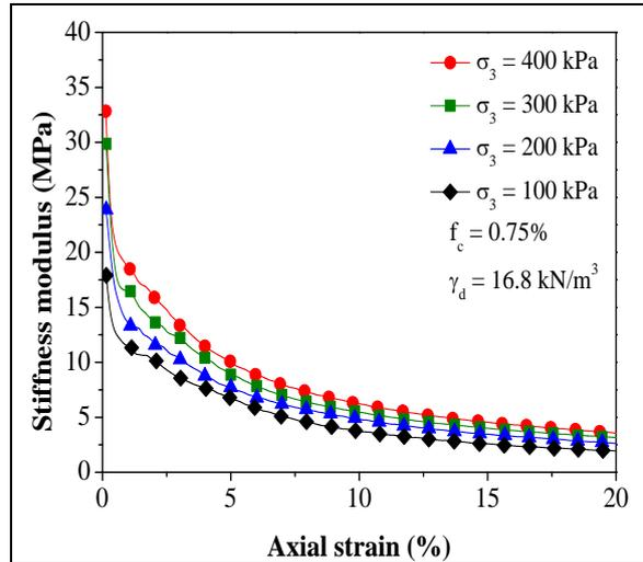
Figure 9 Effect of confining pressure on stiffness modulus
