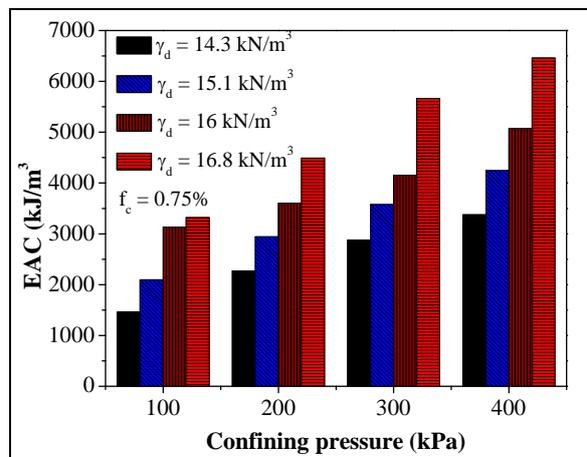
Figure 12 Effect of dry unit weight on EAC
