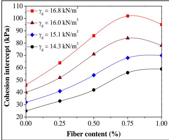
Figure 7 Combined effect of dry unit weight and fiber content on induced cohesion
