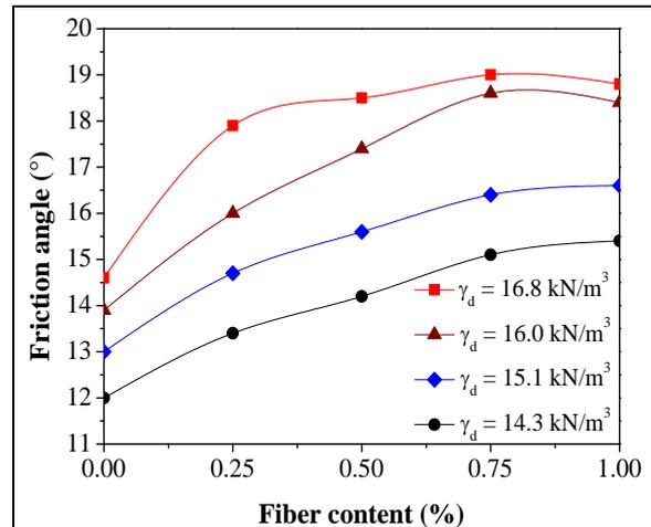
Figure 6 Combined effect of dry unit weight and fiber content on friction angle
