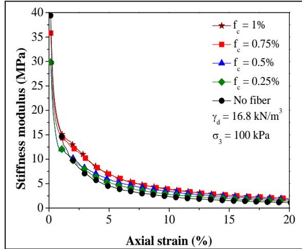
Figure 8 Effect of fiber content on stiffness modulus response
