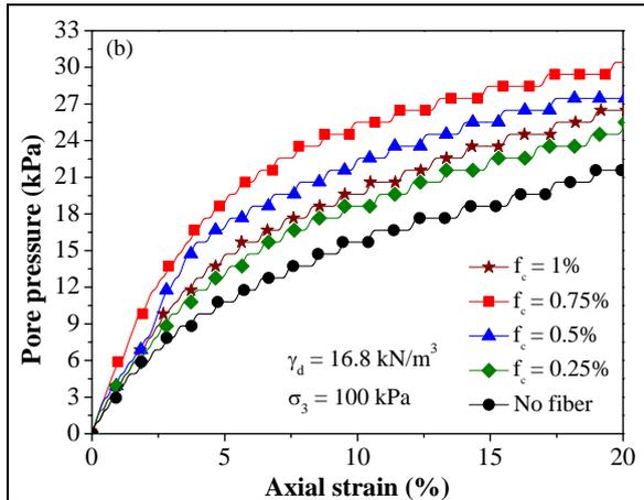
Figure 1 Effect of fiber content on (a) stress-strain and (b) pore pressure response
