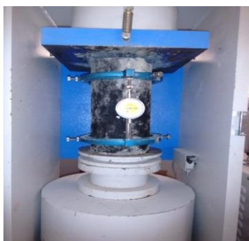
Fig. 4 Compressive modulus of elasticity Test on HCFA GPC
