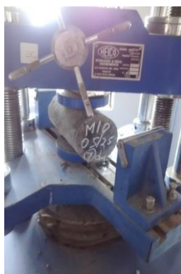
Fig.3 Split tensile strength test
